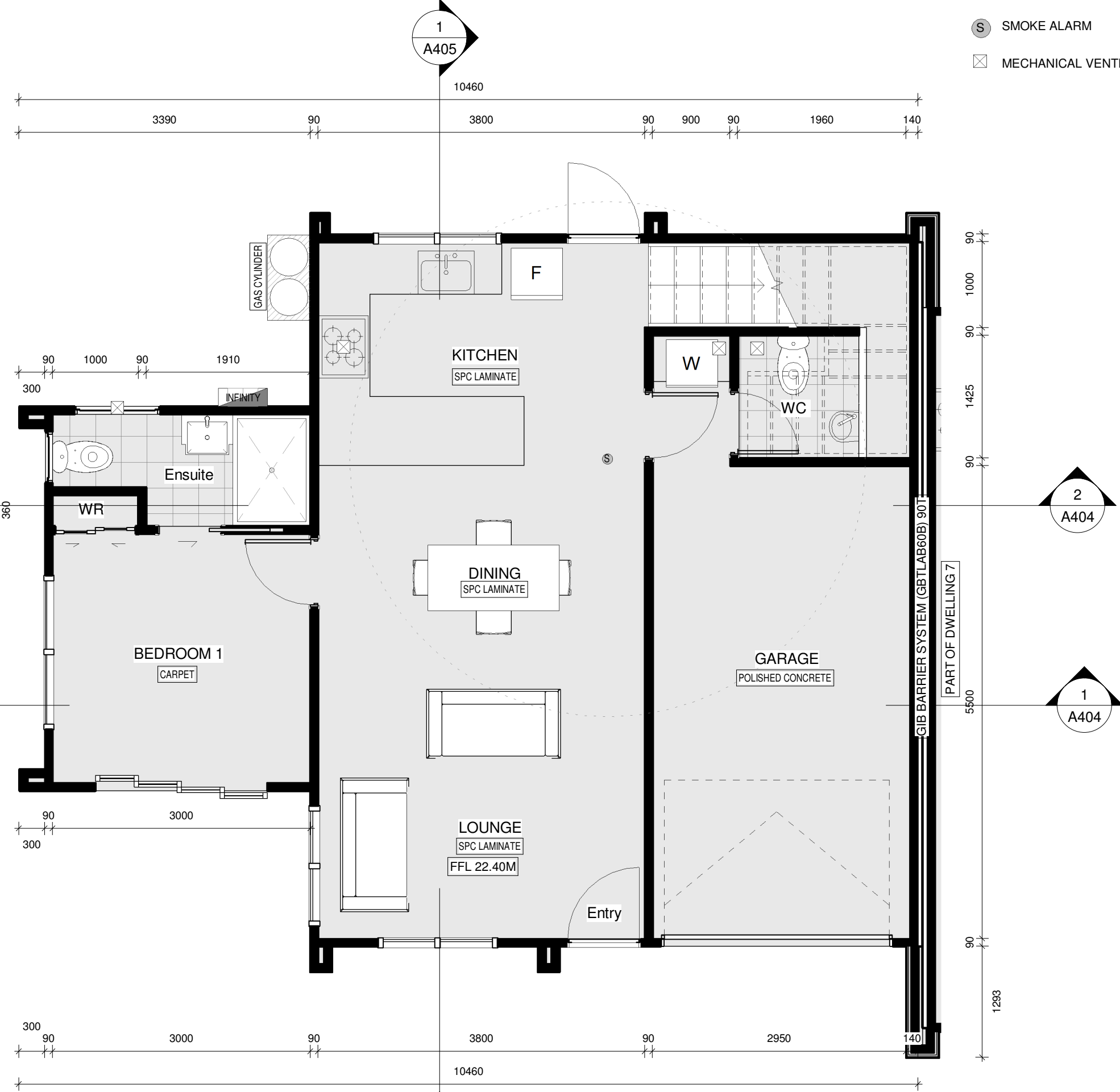
1 LOT 6 - PROPOSED GROUND FLOOR PLAN A205 1 : 50 @ A3 LOT 6 GROUND FLOOR: 73SQM FIRST FLOOR: 73SQM TOTAL: 146 SQM
